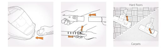
**NOTE:** The Turbobrush, hard floor tool, crevice tool, upholstery tool and dusting brush can all be attached directly to the telescopic tube or hose handle. The TurboTool should be attached via the supplied connector.
