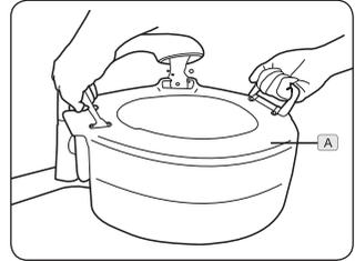
Remove clean water tank (A) from inside the dirty water tank and fill with warm (max 40°C) water to point indicated on the tank. Add 1 capful of Vax Carpet Cleaning solution per litre of water (unless otherwise stated on the bottle).
