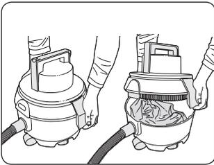
Turn off the vacuum cleaner and unplug it from the mains. Remove the hose. Unclip the retainer clips on either side of the vacuum cleaner and lift off to gain access to the dust bag compartment.
