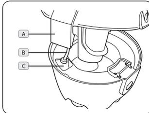
Replace motor container (A) ensuring that the solution pump hose (B) is aligned with the hole in the clean water tank (C) so that it goes inside when the motor container is clipped back into position.
