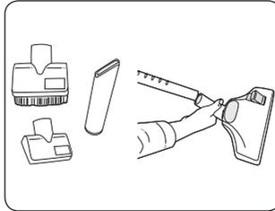
The accessories can also be attached to the extension tubes for extra reach. Remove the combination floor tool and push on the desired accessory.
