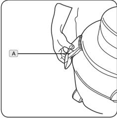
Unclip Container Release Clips (A) on both sides of machine.
