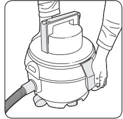
Replace the motor top, ensuring that the dust bag is not trapped. Ensure the motor top is secured to the base with the two clips.
