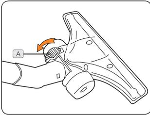
1. On the Fibreflow wash head ensure that the rocker switch (A) is towards the back of the head to allow water to flow through the head.
