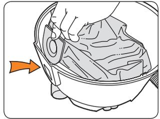
Dispose of the full dust bag and insert a new dust bag back into the vacuum cleaner aligning the front of the dust bag with the inlet slots.
