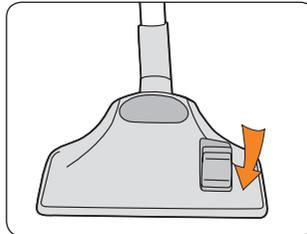
For carpet cleaning, press the rocker switch on the combination floor tool as shown to raise the brushes.
