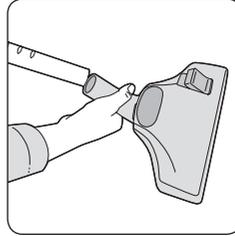
Fit the combination floor tool by pushing on to the extension tube.
