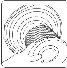
Fit the pleated pre-motor filter by pushing and lightly twisting the filter on the motor top.
