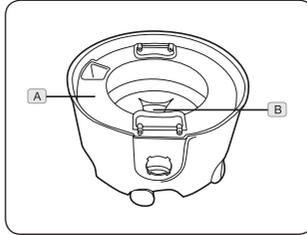
Lift off motor container and remove filter assembly. Remove the plug from the solution intake port and replace the solution connector tube. The machine can be used for washing by placing the clean water tank (A) back inside the dirty water tank (B).
