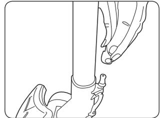
Push the second extension tube into the wash head to be used and push the end of the solution tube onto the connection port on the Wash Head / Upholstery Tool.
