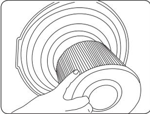
Remove the filter by twisting gently. This will release it from the motor housing.
