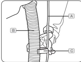
After wrapping the tube around the hose, affix solution tube (A) to hose (B) using clips provided (C) to hold it in place.
