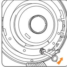
Remove the solution connector tube by turning anti-clockwise by 90 degrees. Store in a safe place.
