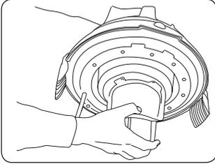
Remove the motor top from the unit, turn on its side and remove the float housing in an anti-clockwise direction to unscrew.
