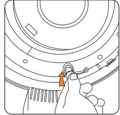
Fit the plug to the solution intake port.
