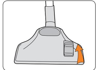
For hard floor cleaning, press the rocker switch on the combination floor tool as shown to lower the brushes.
