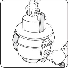
Insert the flexible hose into the inlet on the main body of the vacuum cleaner. Push in and twist clockwise a quarter turn until tight.
