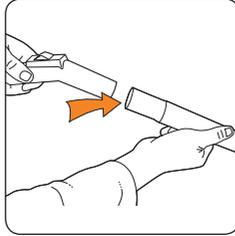
Push the extension tubes onto the end of the handle.
