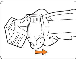
7. Stop the washing solution flowing. To stop the flow, pull the black collar on the wash tool backward.
