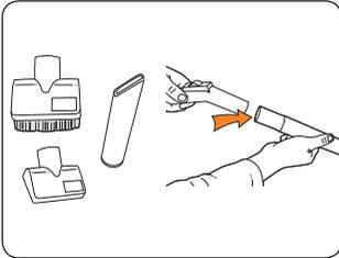
The accessories can be attached directly to the handle by removing the extension tubes and pushing in the desired accessory.
