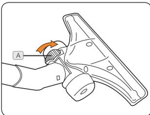
3. Stop the solution flow by moving the rocker switch (A) to the forward position on the Fibreflow wash head. This will prevent water flow, allowing excess water to be removed from the section just washed.
