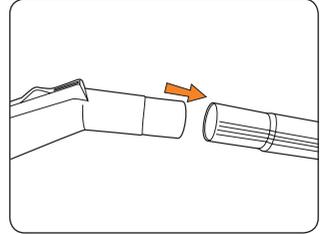
Push one end of the extension tube into the handle of the hose.
