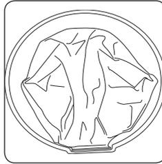
Fit the dust bag by aligning the front of the dust bag with the inlet slots, and position the dust bag to fill the inside of the base.
