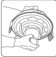
Remove the motor top from the unit, turn on its side and remove the float housing in an anti-clockwise direction to unscrew.
