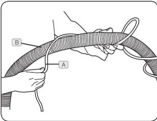
Wrap solution tube (A) around hose (B). Ensure that the solution tube is wrapped loosely enough to allow the solution to flow freely through the tube.
