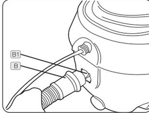
Push hose connector (B) firmly into hose connection port (B1). Twist to the right until hose connector locks into place.
