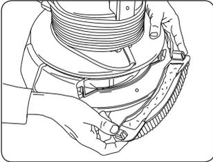
Remove the filter housing at the back of the machine.
