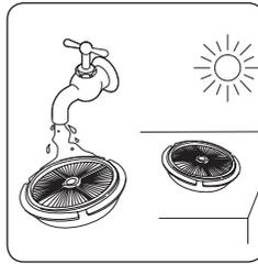
Gently tap the filter against the side of the rubbish bin to remove excess dirt. The filter may then be rinsed in cool water. Allow to thoroughly air dry before replacing.
