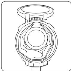
Unclip the retainer clip on the top of the vacuum cleaner and lift up to gain access to the dirt container department.
