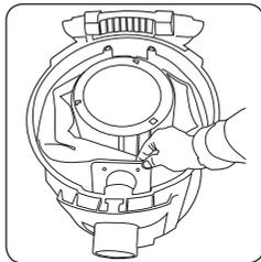
Lift out the full dust bag and dispose of it. Insert a new dust bag into the vacuum cleaner. Align the front of the dust bag with the air entrance.
