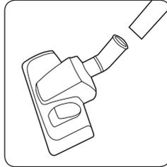
Fit the combination floor head by pushing onto the extension tube.
