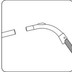
Push the extension tube on to the end of the handle. The extension tubes can be used together to lengthen or shorten by using one section of the extension tube as required.
