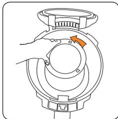
The pre-motor filter is found in the centre of the dirt container. Rotate the filter retaining disc anti-clockwise to gain access to the filter.
