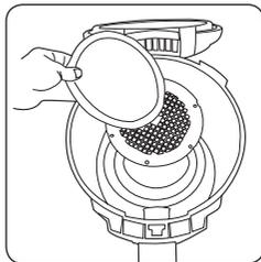
The pre-motor filter can be lifted out.
