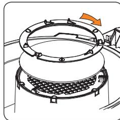
Replace with a new filter inside and turn the retaining disc clockwise to secure.
