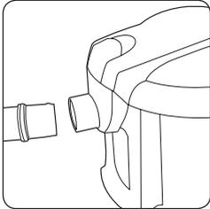
Insert the flexible hose into the inlet on the main body of the vacuum cleaner.
