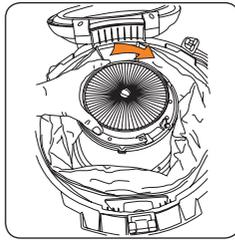
The HEPA pre-motor filter is found in the centre of the dirt container.
