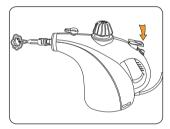
Press steam trigger to release steam.
