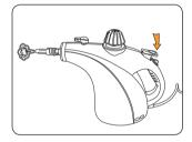
Press steam trigger to release steam.
