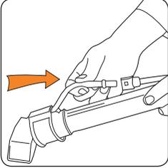
Attach the upholstery wash tool directly onto the handle of the hose and wrap the excess solution tube around as necessary.
