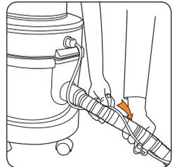
Press down on clips to secure.
