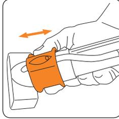
To start water and solution flow, push the collar on the wash tool forwards.
