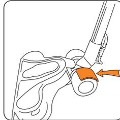
To suck up excess water push the rocker switch to the front.
