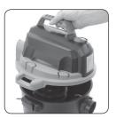
Place the top motor housing cover onto the main tank and secure into position with the two retaining clips.
